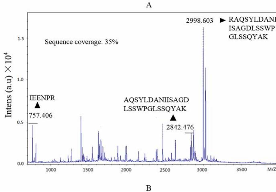
**Fig. 9** MALDI-TOF mass spectrometry analysis of the purified recombinant protein. The amino acid sequence of the recombinant fusion protein BmILP is displayed in panel A with the mass spectrometry identified sequences underlined. The identified sequences were labeled on corresponding mass spectrometry peaks in panel B.
