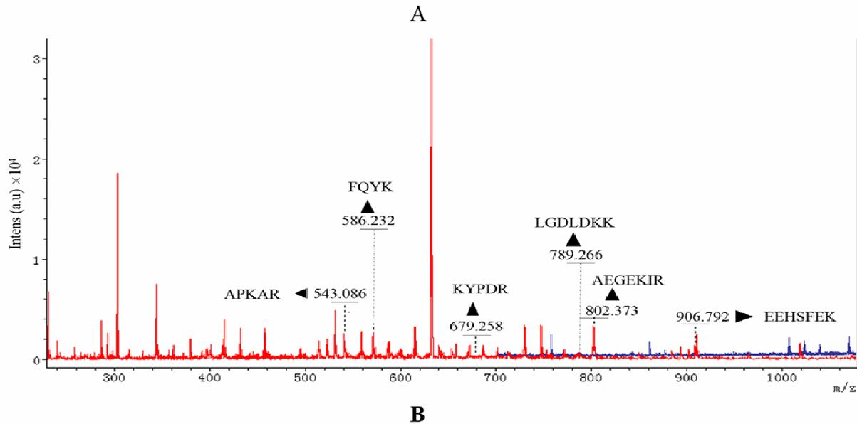
**Fig. S2** Mass spectrometry analysis of the prey protein from lane A5 in the Fig. 10. The amino acid sequence of the autophagy-related proteins Atg8 of the silkworm is displayed in the figure A. The peptides that were identified by mass spectrometry were labeled on top of the peaks in the figure B and underlined for the corresponding sequence.
