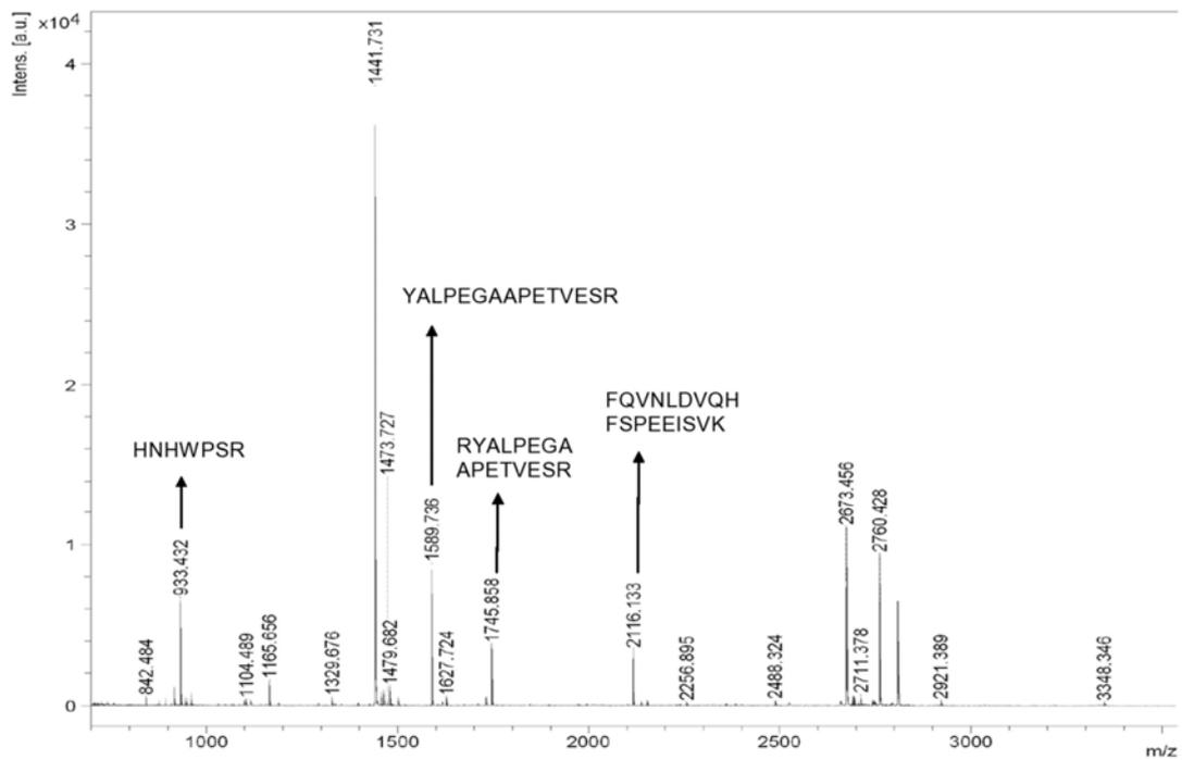
**Suppl. Fig. 6** MALDI-TOF-MS analysis of tryptic fragments of spot 6. The 2DE spot was cut into small pieces, subjected to overnight in-gel trypsin digestion, and then prepared for analysis by MALDI-TOF-MS. Peaks at 933.432, 1589.735, 1745.858, 2116.133 corresponded to the predicted tryptic fragments of HSP 20.8.
