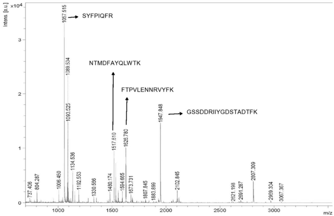
**Suppl. Fig. 5** MALDI-TOF-MS analysis of tryptic fragments of spot 4. The 2DE spot was cut into small pieces, subjected to overnight in-gel trypsin digestion, and then prepared for analysis by MALDI-TOF-MS. Peaks at 1057.515, 1517.610, 1626.780 and 1947.848 corresponded to the predicted tryptic fragments of 29 kDa low molecular weight lipoprotein.
