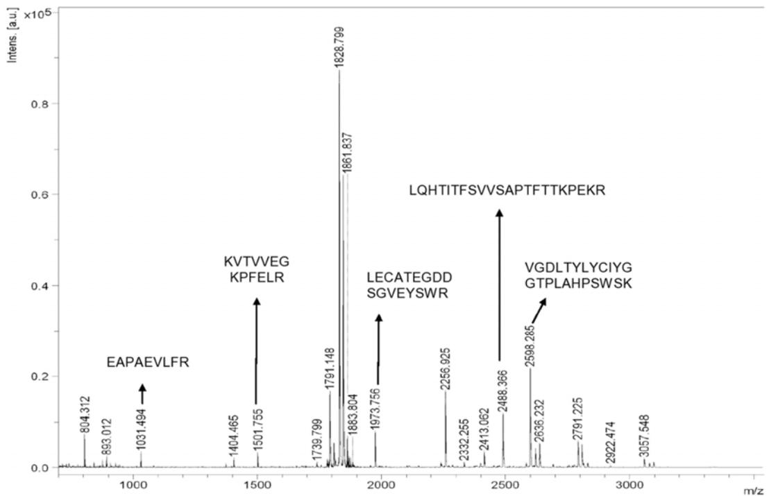
**Suppl. Fig. 4** MALDI-TOF-MS analysis of tryptic fragments of spot 3. The 2DE spot was cut into small pieces, subjected to overnight in-gel trypsin digestion, and then prepared for analysis by MALDI-TOF-MS. Peaks at 1031.494, 1501.755, 1973.756, 2488.366 and 2598.285 corresponded to the predicted tryptic fragments of Hemolin.
